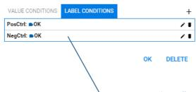
This "Label condition" means that both the controls ("PosCtrl" and "NegCtrl") must be satisfied ("OK"), in order to assign the label "Present" to the sample.
