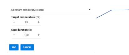
Use this option to insert a constant temperature step. Use it to include initial denaturation/polymerase activation step. Set the conditions for temperature and length.
