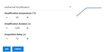
Use this option for LAMP (Loop-mediated isothermal amplification) assays. Set the conditions for:
